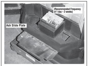
Figure 45 - Using the Ash Slide Plate
